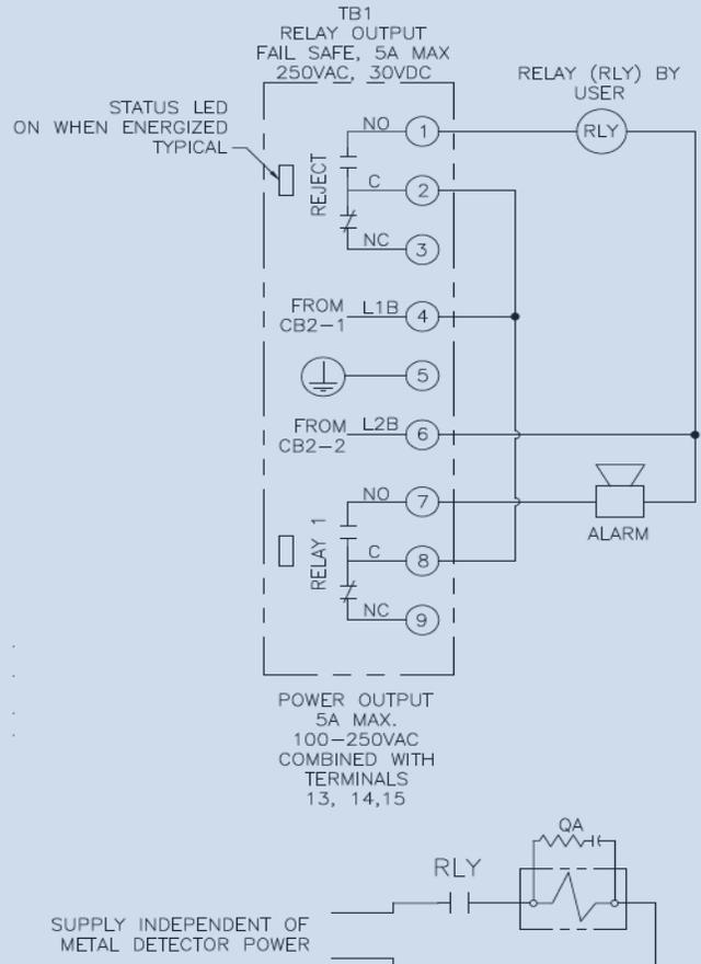
Figure 14: Output connection examples
