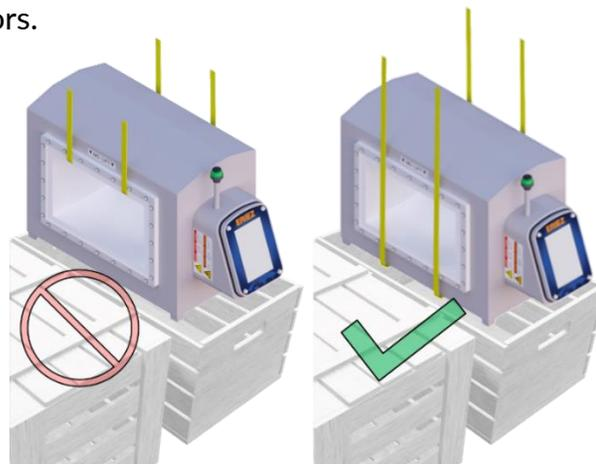
Figure 1: Metal detector handling instructions
