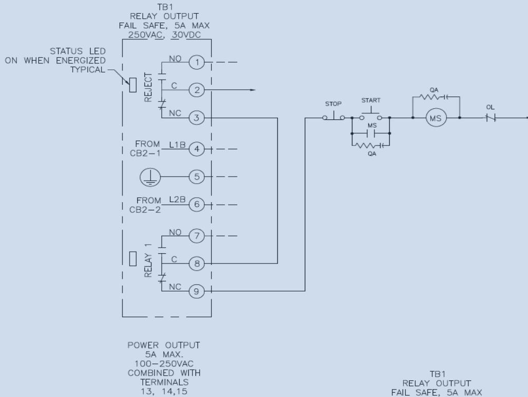
REJECT & ALARM DEVICES POWERED BY THE INTERNAL SOURCE MUST BE RATED AT THE SAME VOLTAGE AS THE INPUT SUPPLIED TO THE METAL DETECTOR
