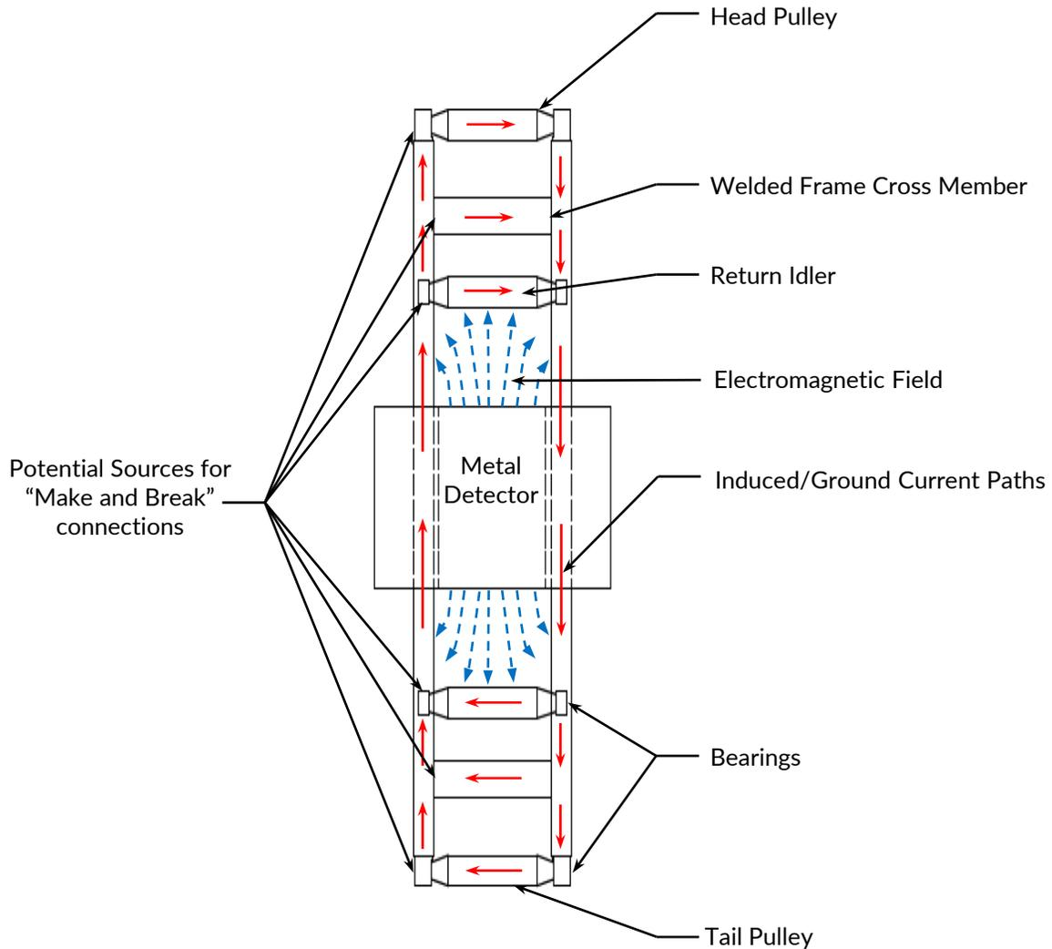
Figure 4: Potential sources for “Make and Break” connections
