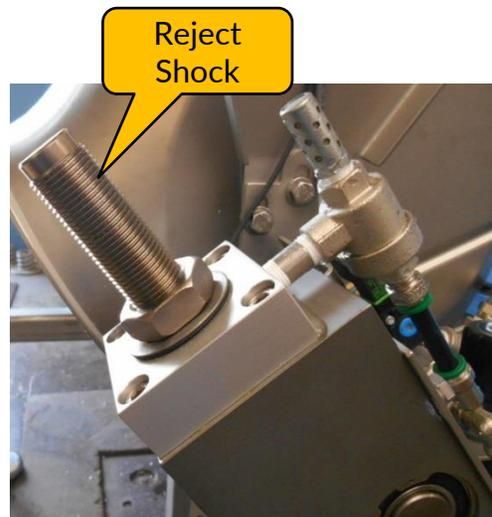
Actuator shock installed
