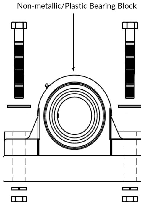
**Figure 7: Recommended method for insulating bearing block**
