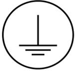
For continued compliance with electrical safety standards, the protective earth connection from the power source must be connected directly to the protective terminal on the wall of the enclosure. This is required to be the FIRST connection to the terminal, and secured with a star lock washer and nut, independent of any other connections to the terminal.
