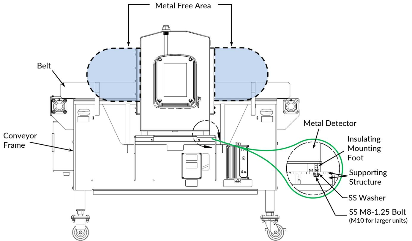
**Figure 9: Metal free area and mounting feet**
