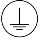
For continued compliance with electrical safety standards, the protective earth connection from the power source must be connected directly to the protective terminal on the wall of the enclosure. This is required to be the **FIRST** connection to the terminal, and secured with a star lock washer and nut, independent of any other connections to the terminal.
