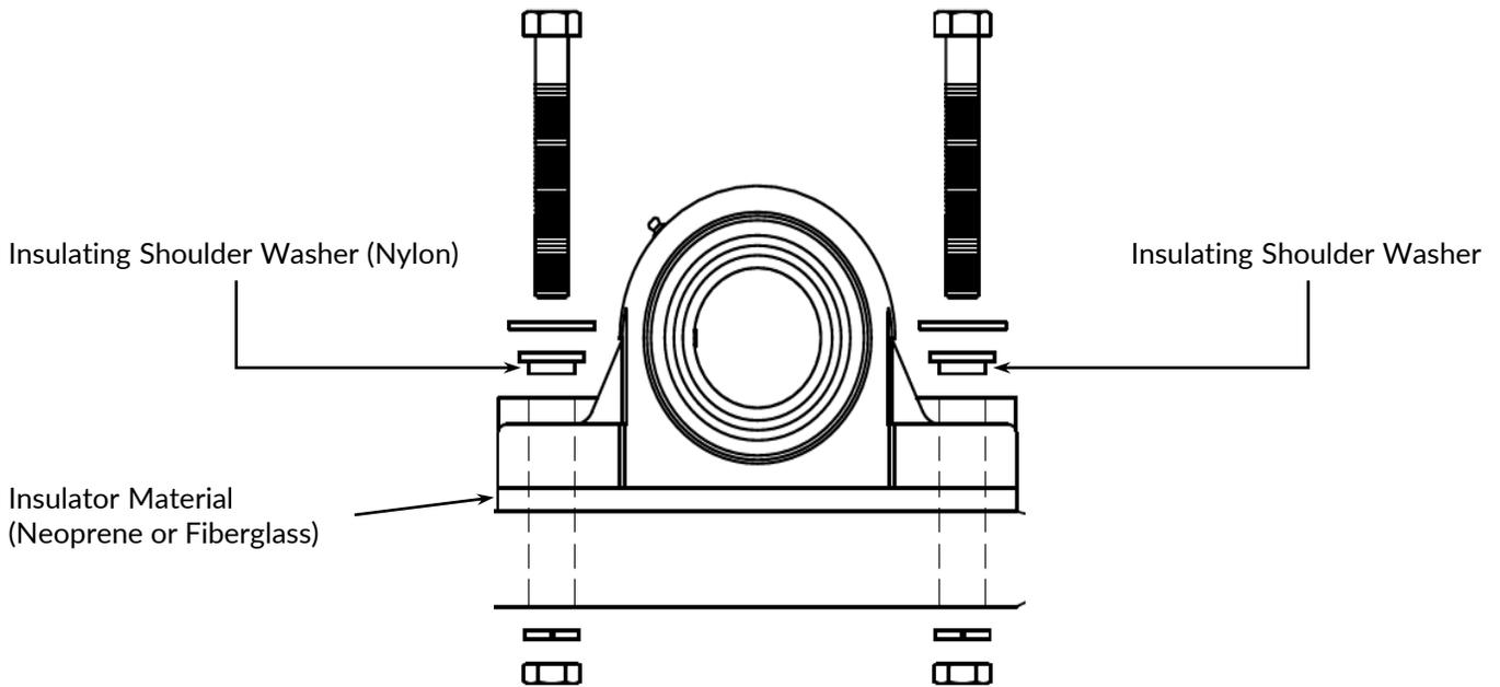
**Figure 6: Bearing block on conveyor frame**
